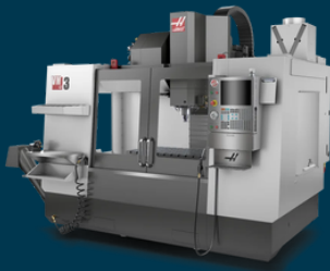
HAAS VM 3 X: 1016 mm No. of Y: 660 mm machines: Z: 635 mm 1
