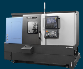
DOOSAN LYNX 2100LYB X: 205 mm No. of Y: 105 mm machines: Z: 560 mm 1
