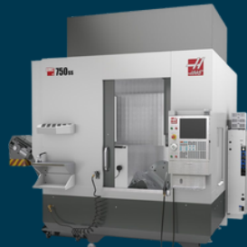
HAAS UMC 750ss X: 762 mm No. of Y: 508 mm machines: Z: 508 mm 2
